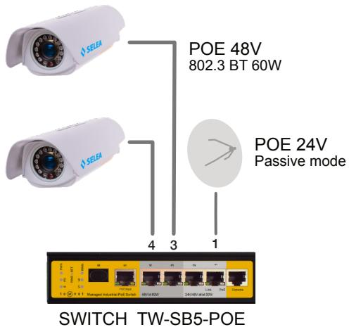
To correctly power the Selea Targa 850 cameras, connect them to ports 3 or 4 (802.3 BT 60W) of switch managed TW-SB5-POE
